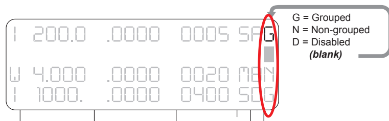
Fig. 14—The Group field appears in the far right column of the display. In this example, the first and last channels are grouped, the second channel is disabled, and the third one is not grouped.
