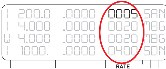
Fig. 11—Place the cursor in the rate field of a channel and use the keypad to enter the desired rate value for the infusion or withdrawal.
