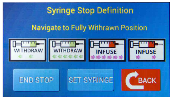
Fig. 30—The Syringe Stop Definition screen lets you define the limits of travel for the pump.
