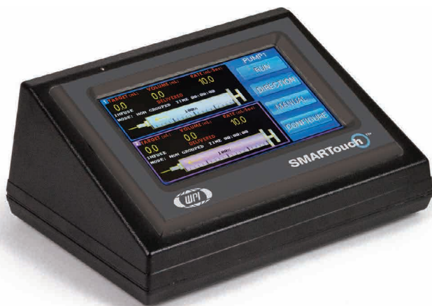
Fig. 5—The MICRO2T touch screen controller shows the command screen.
