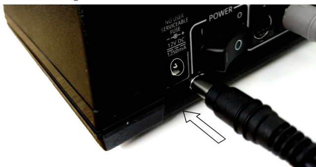
Fig. 16—Connect the power supply to the power port on the controller.
